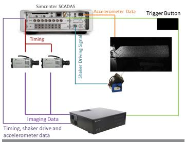
Usage of iX 727 High-Speed cameras for DIC measurements
