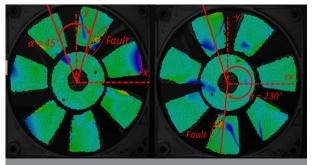
A vibration analysis is made using FFT and the ODS module of MatchID. An FFT analysis on the out-of-plane motion of the defective blade reveals the actual vibration frequency of the blade. This frequency can be used to reconstruct the operational deflection shape of the faulty fan assembly.
