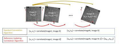
A standard DIC algorithm will perform well up to rotations of around 40 degrees. To comply to larger rotations, a reference updating scheme can be adopted. As such, correlation is not performed w.r.t. the initial reference state, but to the preceding image in the rotation cycle. The total displacement is then achieved by incrementally adding these small-step rotational displacements . Noise might be accumulated as well, but giving the large signal involved this is of minor importance.
