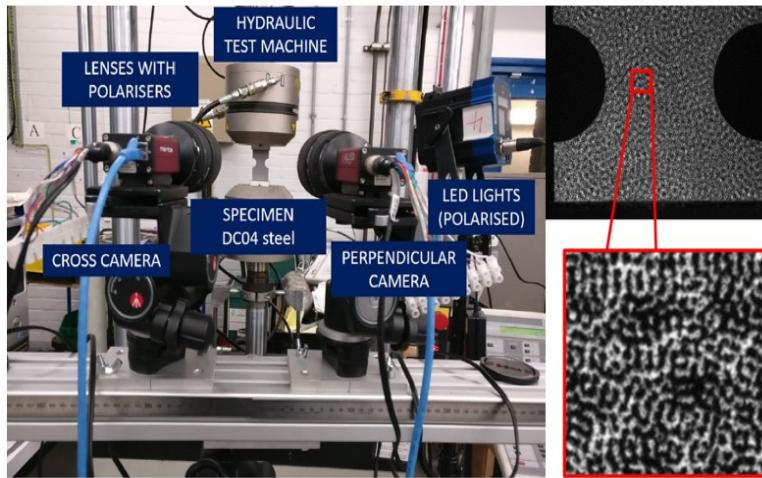
Specimens were water-jet cut out of a cold-rolled sheet of DC04 low-carbon steel alloy with a nominal thickness of 1.5 mm. An optimized speckle pattern was printed on the specimen using a flat-bed printer which provided good consistency and reproducibility. An average speckle size of approximately 65  $\mu\text{m}$  was achieved. Deformation was measured using a stereo-DIC set-up. By setting cross-polarization specular reflection was minimised which
