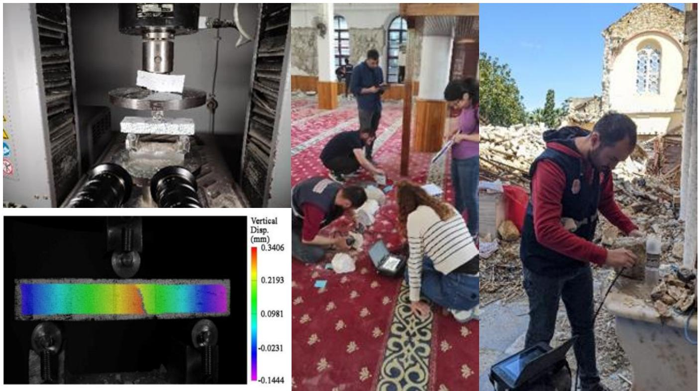
MatchID supports research on the characterisation of the materials of historic stone buildings which were damaged during the 2023 Turkey-Syria earthquakes. The research aims to provide underpinning data to support forensic investigations and restoration projects.
