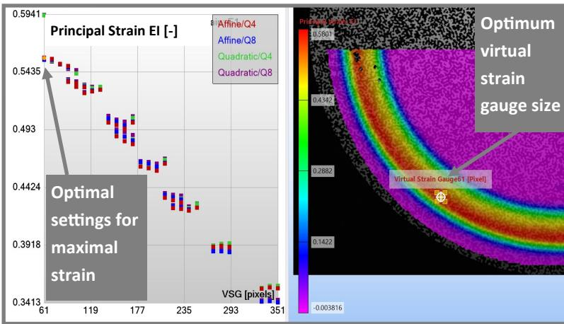
In this study, the aim is to retrieve the DIC settings that generate a maximum and converged strain value. The full-field plot shows the size of the corresponding virtual strain gauge, indicating the actual size of the adopted smoothing area.
