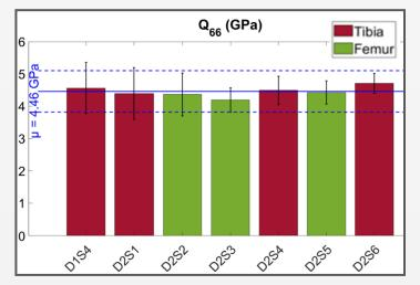
on each side. This opens up the way for much more efficient testing of human bone for which samples are very valuable. It also allows for more accurate sampling of property heterogeneities within a femur or tibia.
