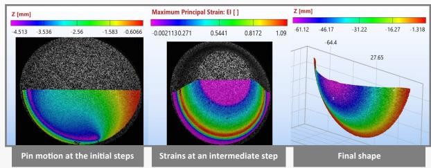
The resulting strain components can be used to derive the thickness distribution of the field by relying on volume conservation. This derivation is made readily available via MatchID's AppStore and can be added to your package via a dedicated plugin. Once the thickness field is obtained, profile sketches are extracted to
