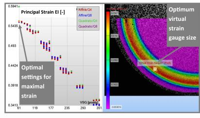
ness, the performance analysis module is used to determine the DIC settings that yield an optimum signal to noise ratio.
